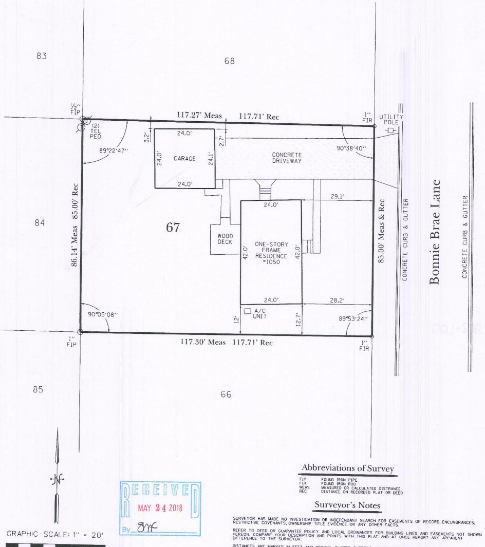
DISTANCES ARE MARKED IN FEET AND DECIMAL PLACES THEREOF, NO DIMENSION SHALL BE ASSUMED BY SCALE MEASUREMENT HEREON. DISTANCES AND/OR BEARINGS SHOWN IN PARENTHESIS (0.00') ARE RECORD OR DEED VALUES, NOT FIELD MEASURED.
